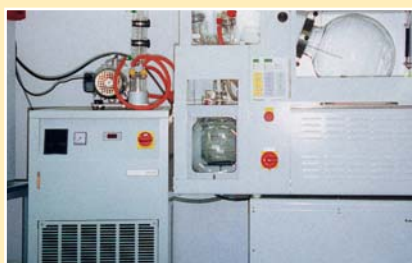
Back-distillation of solvents with a rotary evaporator
