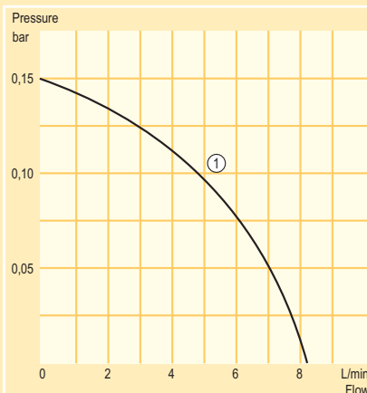
Pump characteristic measured with Kryo 30
